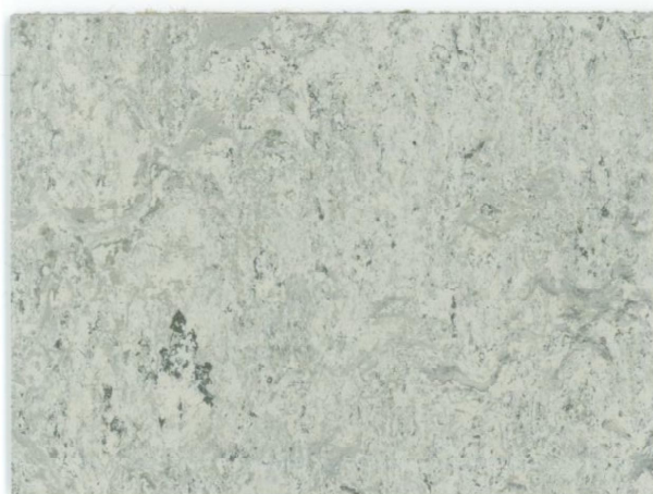
Linoleum Forbo Marmoleum real Farbe 3032, 2,0 mm ca. 10^{10} - 10^{11} Ohm
